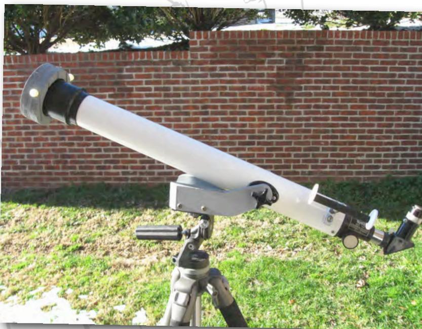
Using a few pieces of scrap wood I made a cell for the Baader film. It would be secured to the scope's dewshield with a couple of nylon thumbscrews. But what about a mount?
